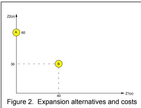
For example, Figure 2 shows two expansion options, A and B, which have to be evaluated under two possible scenarios. The costs of option A for scenarios 1 and 2 are respectively 0 and 60. The costs of B for the same scenarios are 40 and 30.
